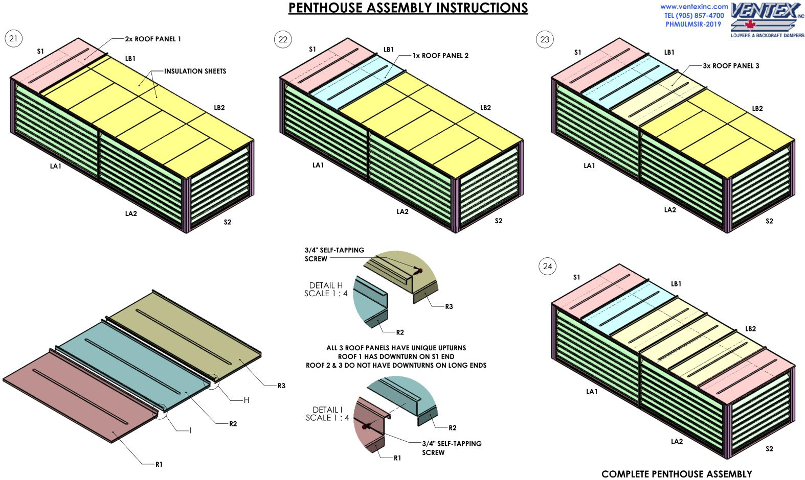
ASSEMBLE THE ROOF PANELS AS SHOWN SCREW THE ROOF FROM SIDES USING 3/4" SELF-TAPPING SCREW
