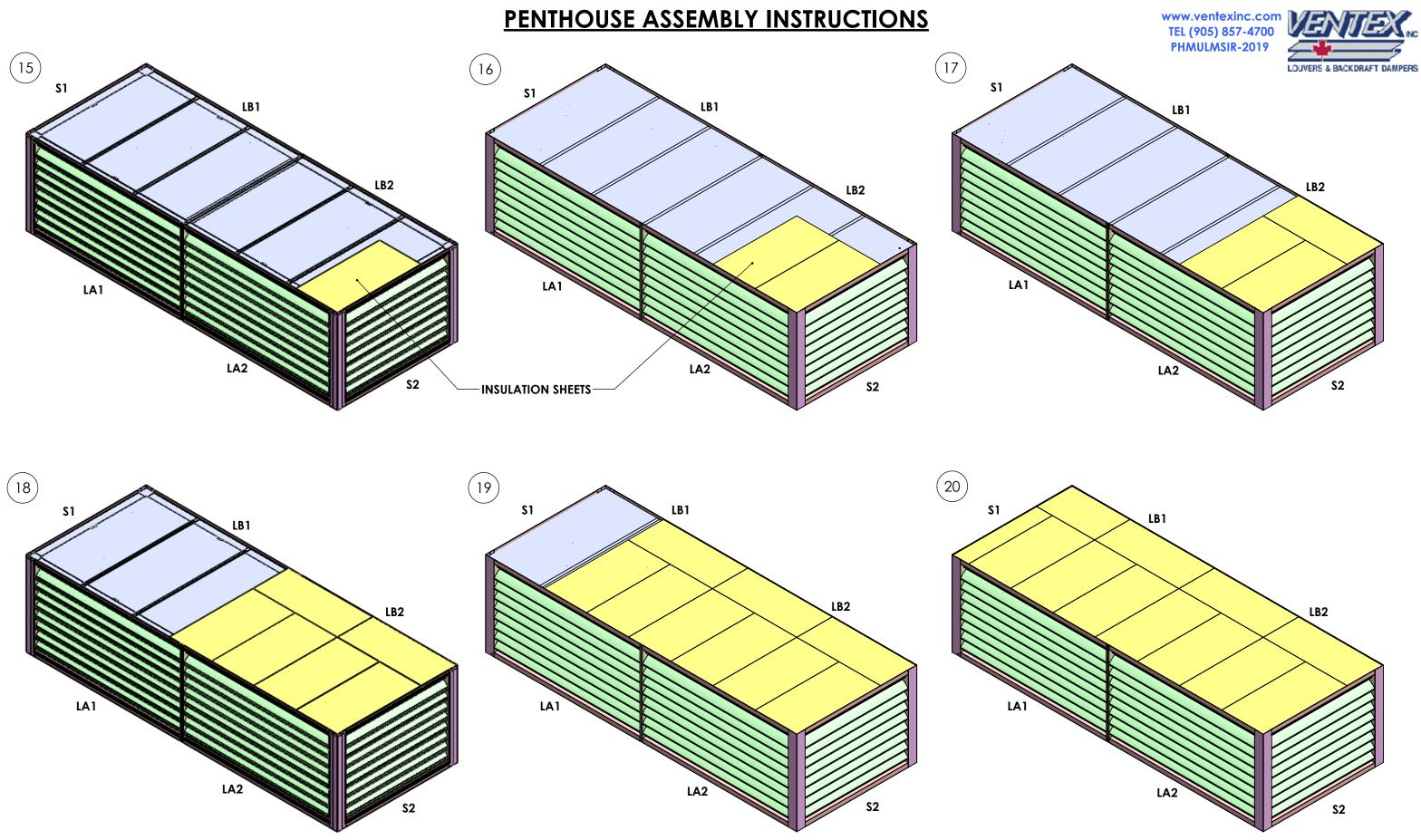
ADD THE INSULATION SHEETS ON TOP OF PERFORATED SHEETS AS SHOWN FOR MAXIMUM COVERAGE
