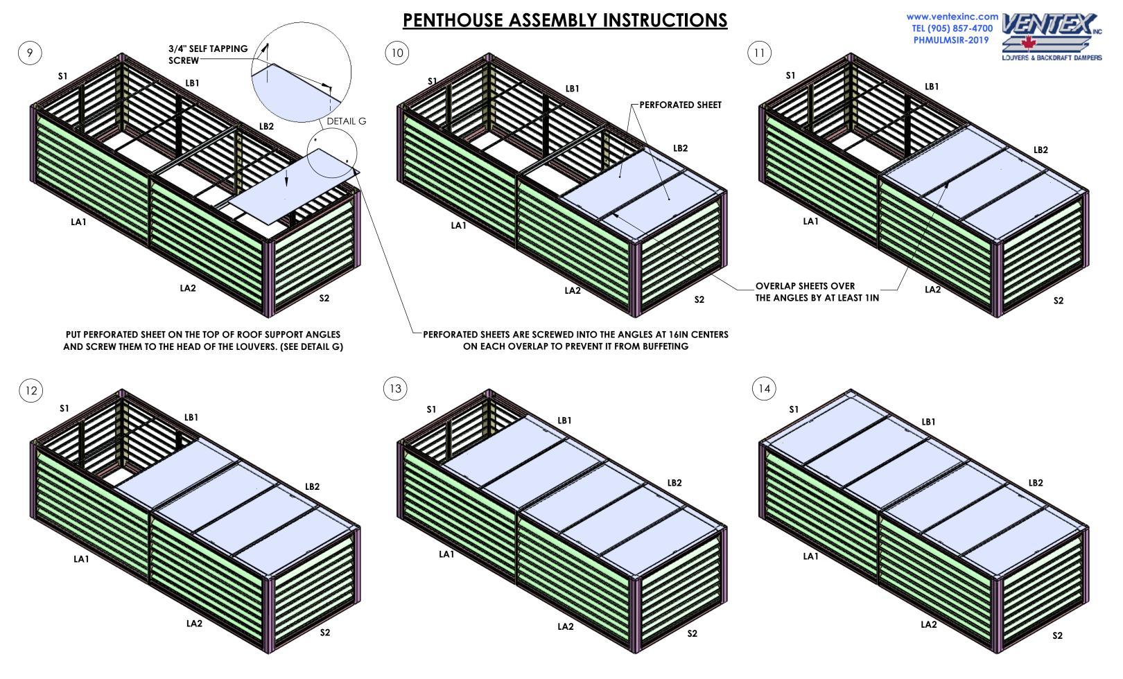
ASSEMBLE THE PERFORATED SHEETS AS SHOWN
